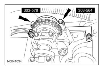
5. **NOTE:** The RH camshaft sprocket is a LH-threaded bolt.
