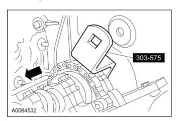
6. Remove the camshaft sprocket bolt and position the RH camshaft sprocket aside.
