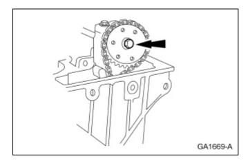
9. Remove the bolt and position the LH camshaft sprocket aside.
